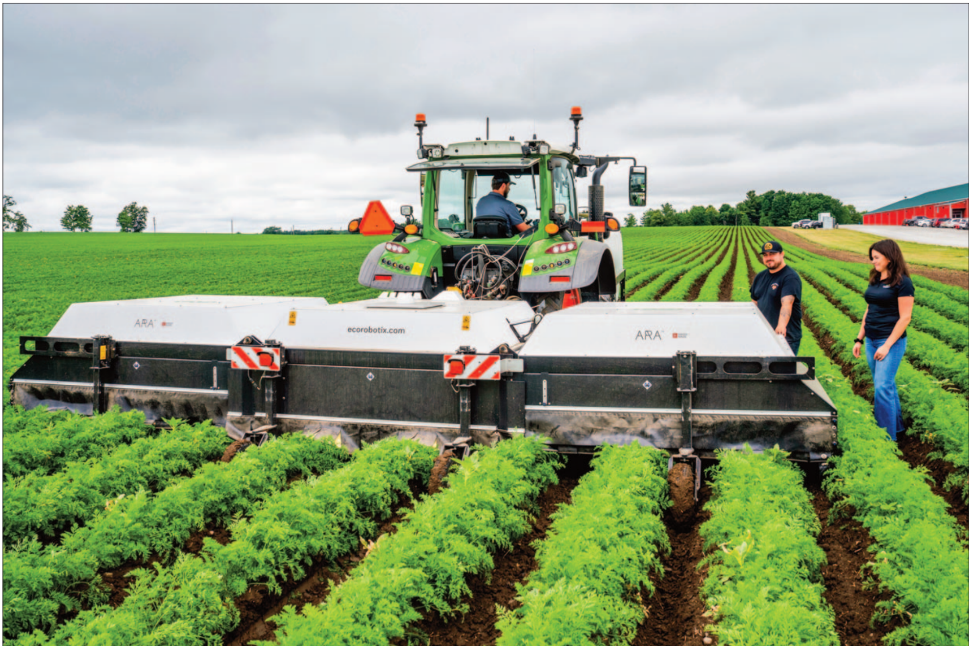
This AI-enhanced sprayer was first used in the field in spring 2025 to spot-spray carrots. The nozzles are programmed to spray only identifiable weeds of up to 16 inches in height. Thanks to input cost reductions, a 100 per cent return on investment is expected in two years. Isaiah Galbraith is in the driver's seat as Alexa Hambly-Galbraith, business operations manager for Gwillimdale Farms, Bradford, Ontario, highlights some of the equipment's benefits to fellow grower Brandon Scholten, Korag Farms. Photos by Paul Novosad.
