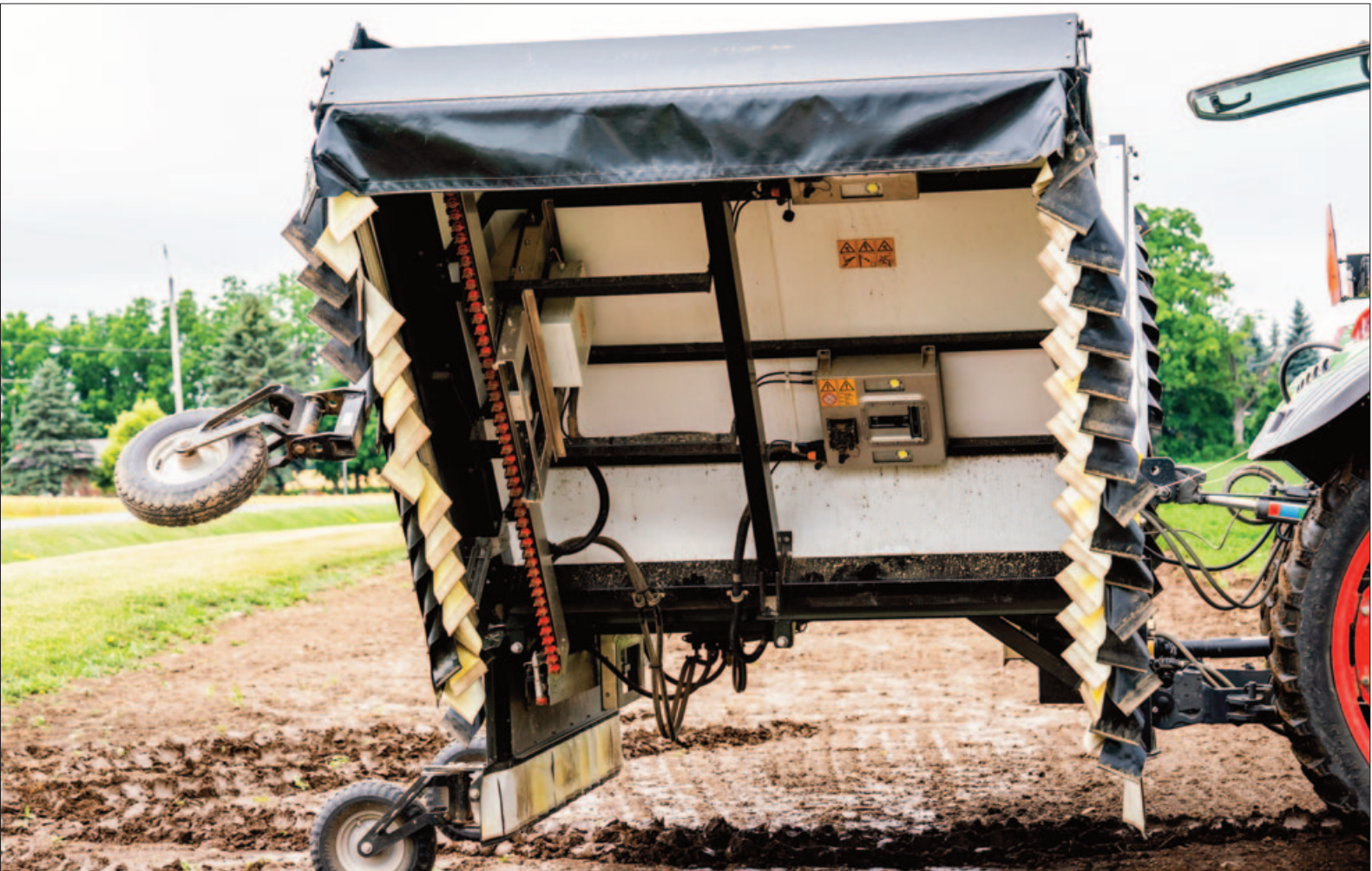
There are 156 high-precision spray nozzles spaced for a four-centimetre spray pattern.
