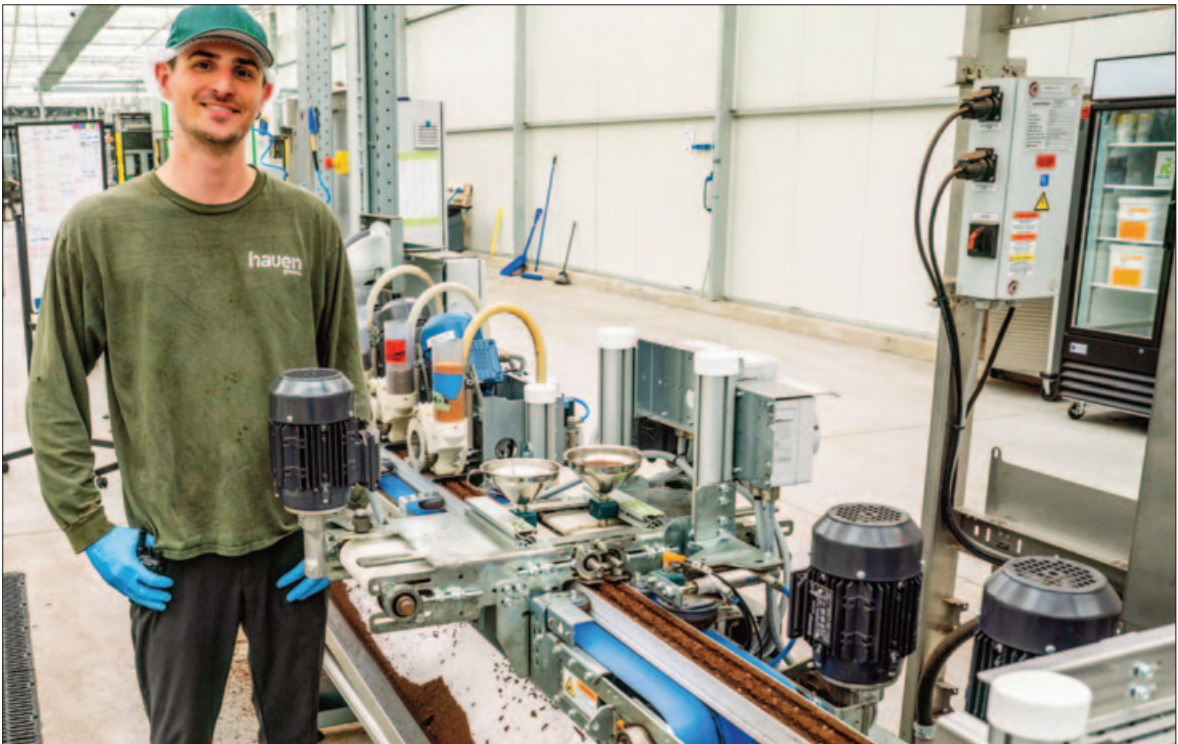
Dominick Dimucci, director of cultivation, stands beside the automated seeding machine. Each seed gutter carries an RFID tag. The data consists of time and date stamp of seeding, the variety, the number of seeds per gutter, the seed lot and the peat lot. Each seed is coated with a mycorrhizial inoculant, binding the seed with its original life partners to enhance rooting.
