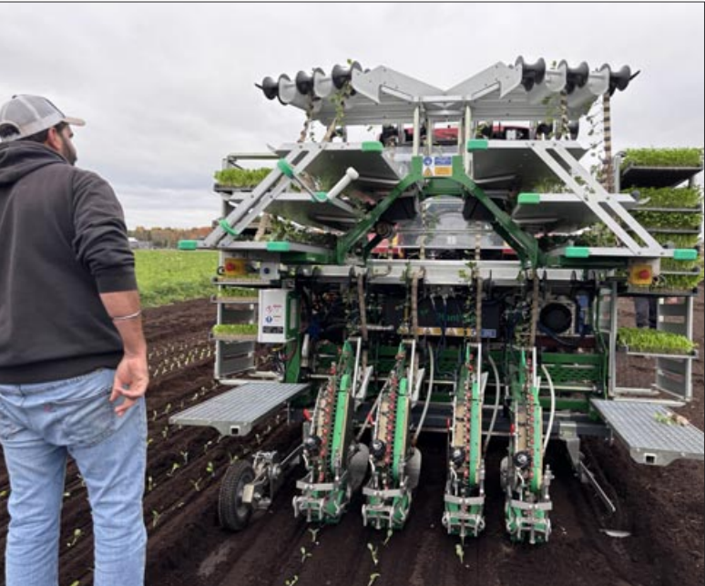
The PlantTape machine travels at two to six km/hour. A diamond pattern is commercially available, allowing up to 50,000 plants per acre in romaine.
